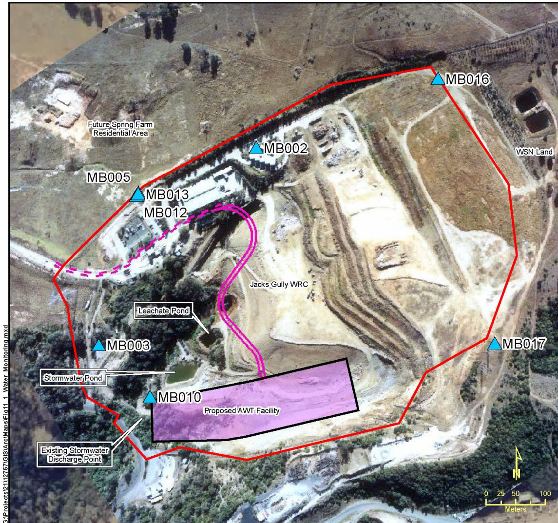
Figure 11-3 Surface water system components and groundwater monitoring points
