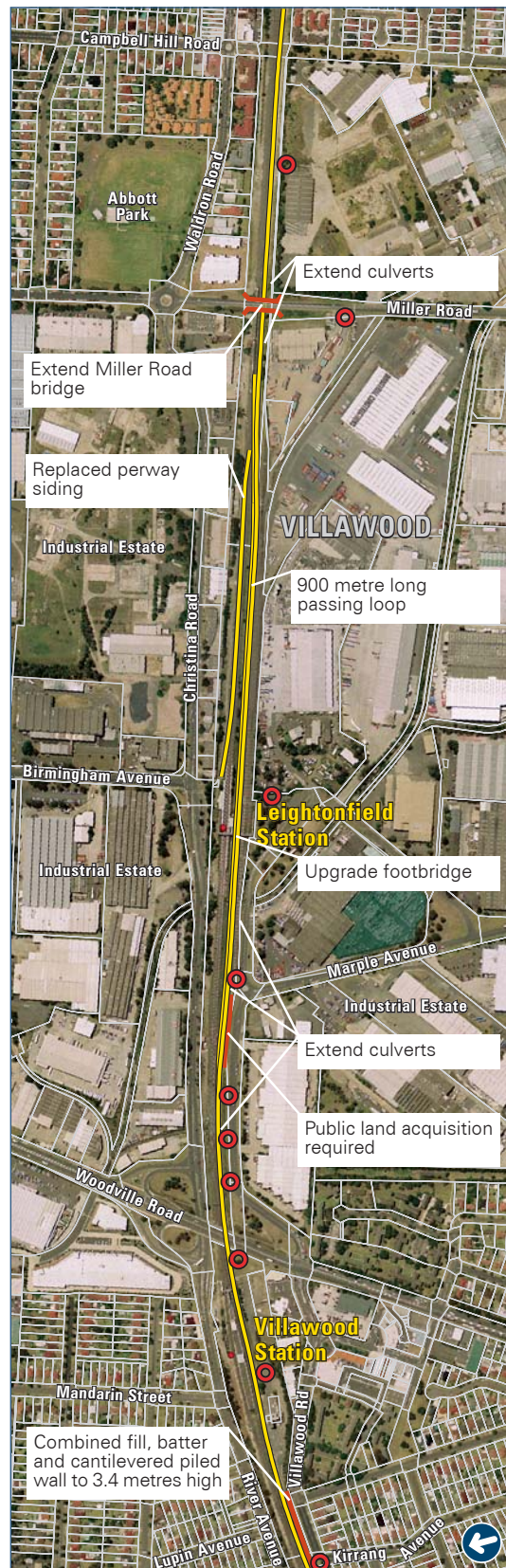
Figure 2g Features of corridor construction
