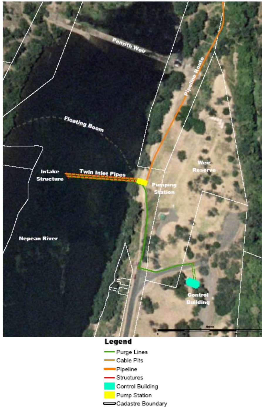
Figure 1-1 Location of the Proposed Pump Station and Control Building
