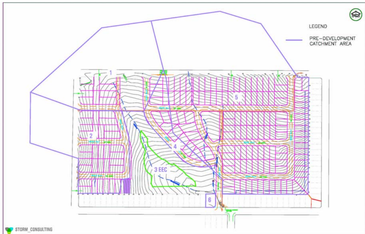
Pre-development subcatchment schematic
