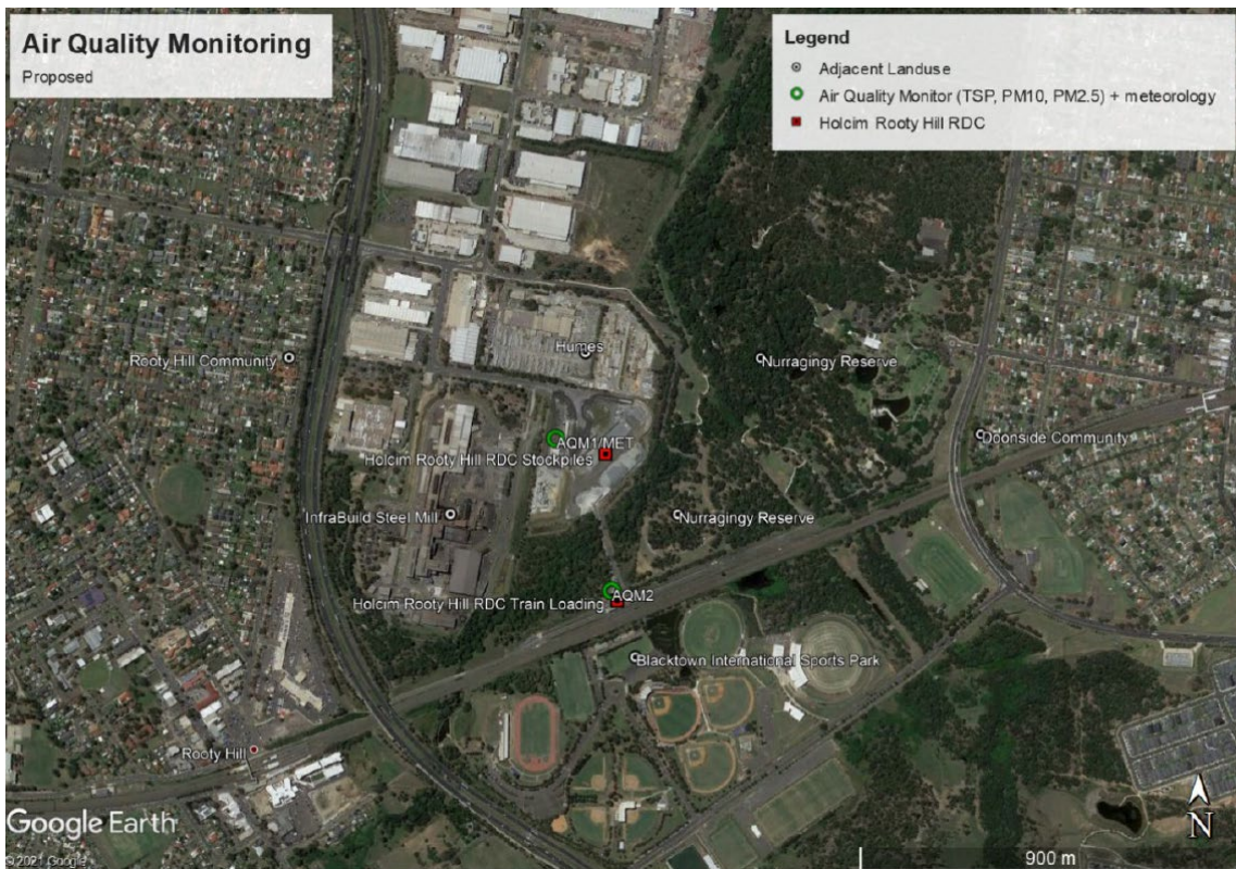
Figure 4: Proposed air quality monitoring program at Holcim RHDC with surrounding land uses, (Ramboll, 13/10/2021, Review of Air Quality Monitoring Locations)
