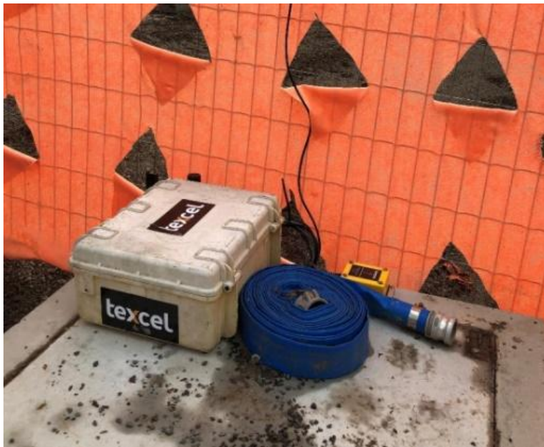
Figure 2 Example of vibration logger
