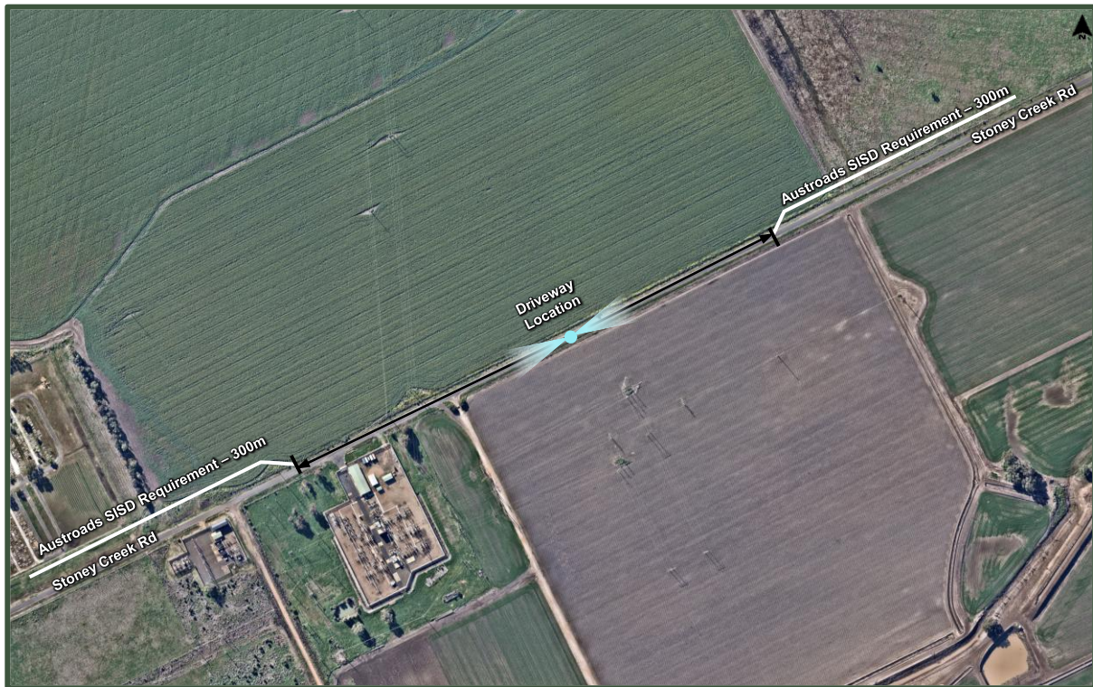
Figure 12 Safe Intersection Sight Distance
