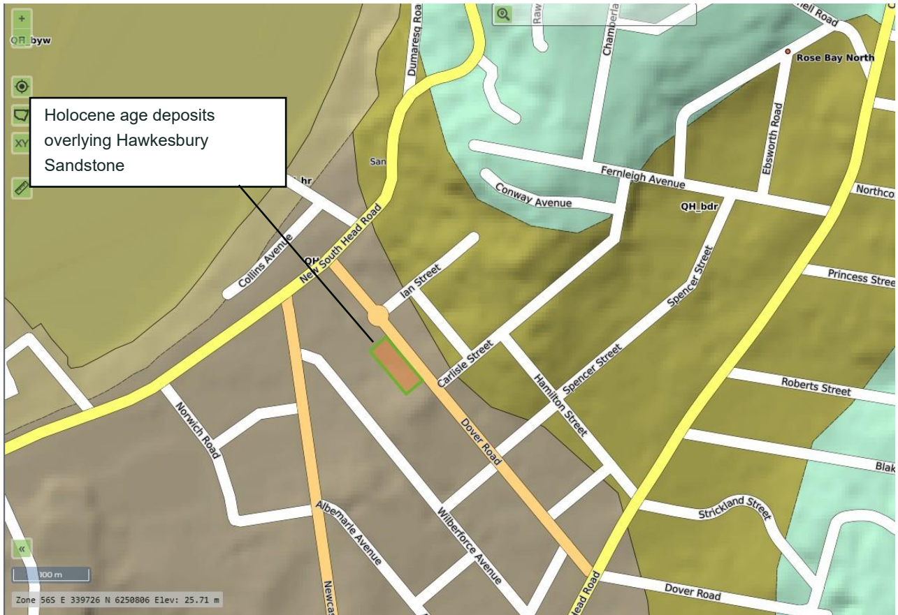
Plate 2-2: Extract of the Minview Seamless Geology Map Showing the site to be covered by Holocene age Coastal & Estuarine Deposits
