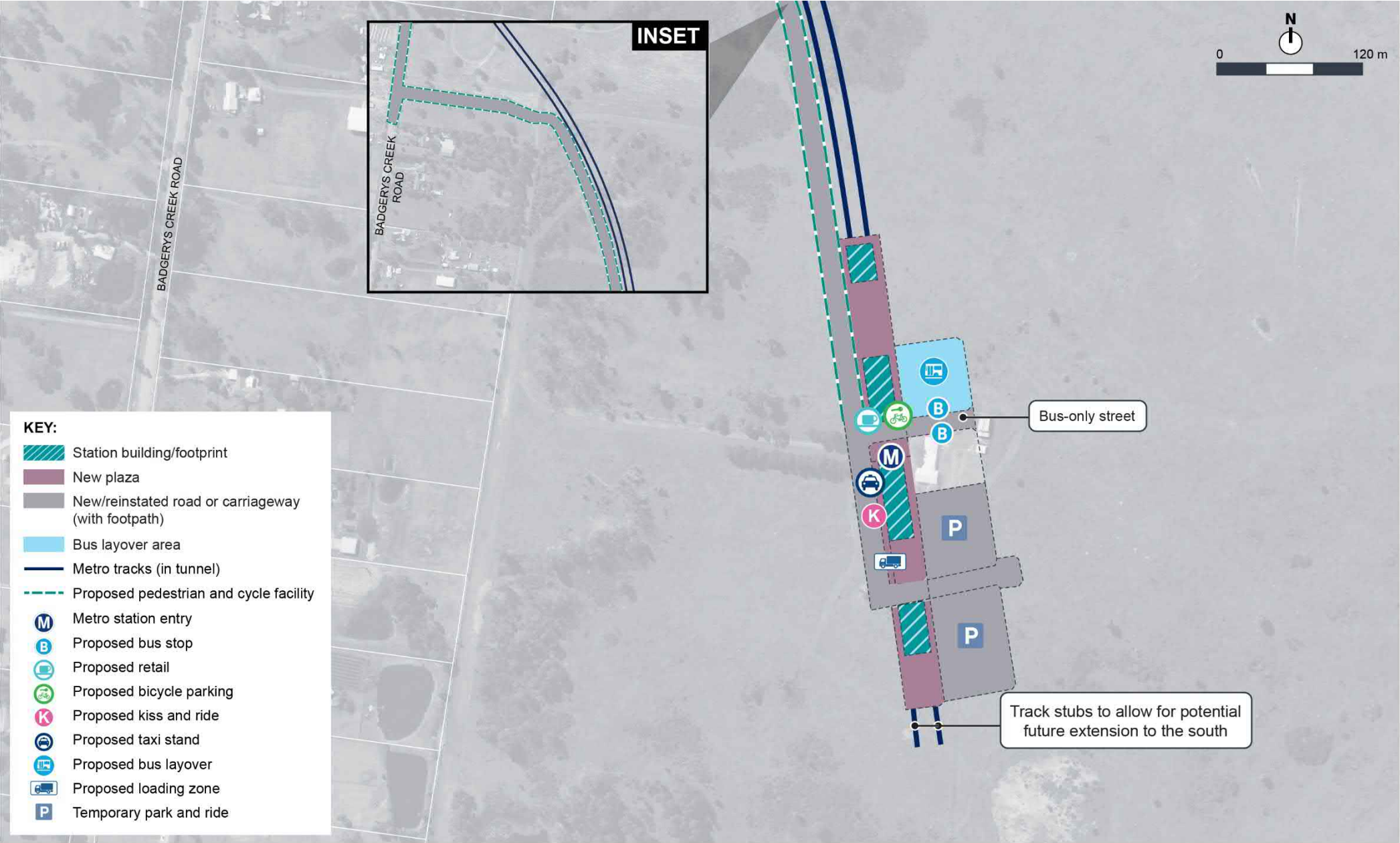
Figure 1-35 Aerotropolis Core Station - Indicative layout and key design elements
