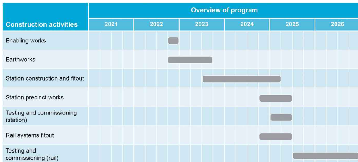
Figure 2-21 Indicative construction program for the Luddenham Road construction site
