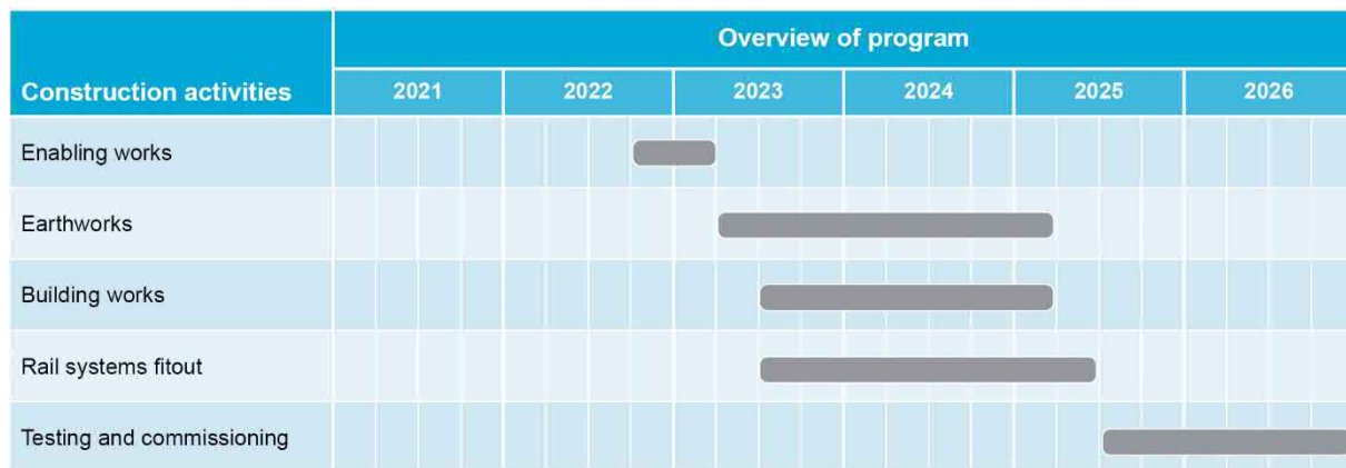
Figure 2-19 Indicative construction program for the stabling and maintenance facility construction site
