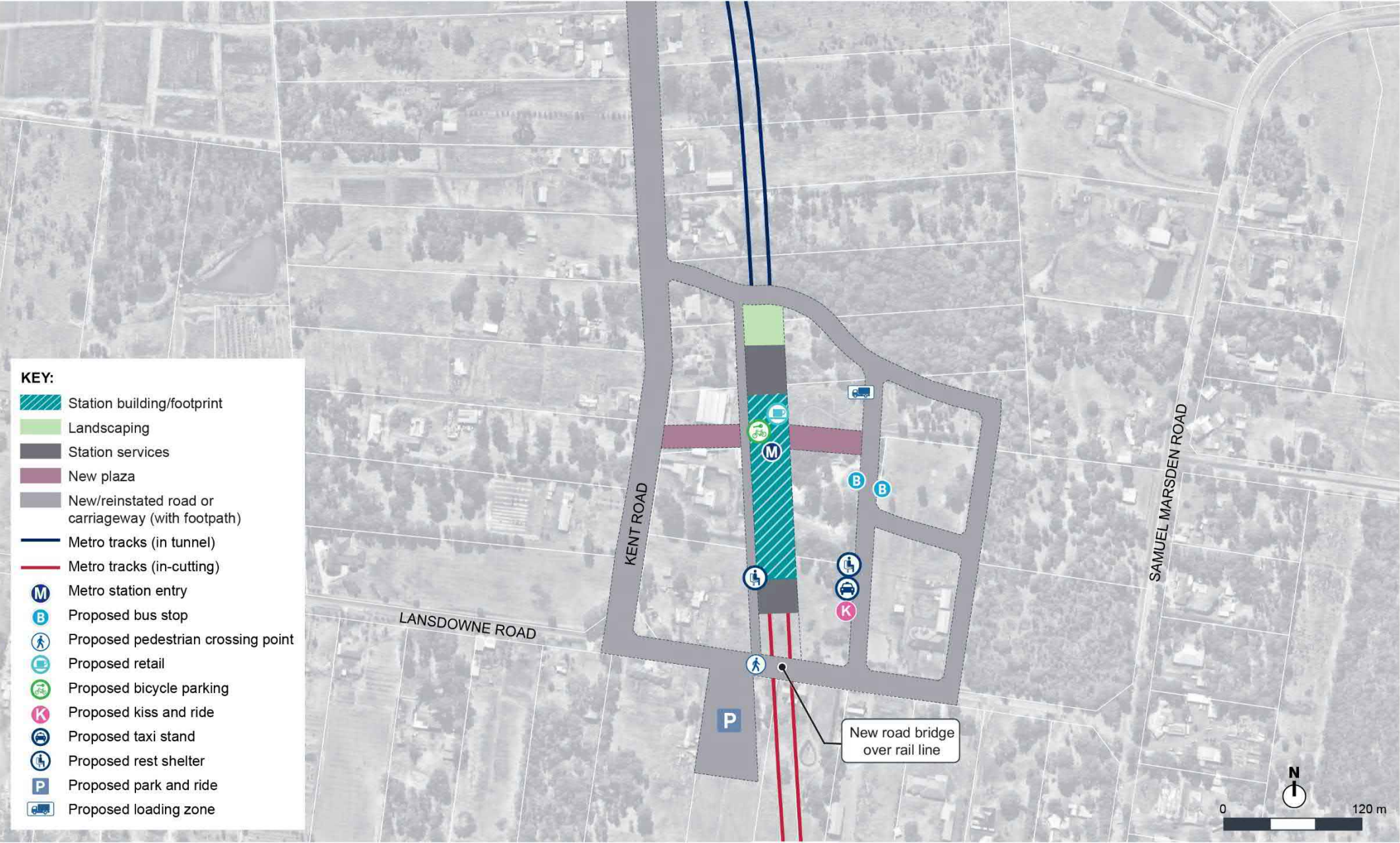
Figure 1-19 Orchard Hills Station - Indicative layout and key design elements Note: Indicative only, subject to design development.
