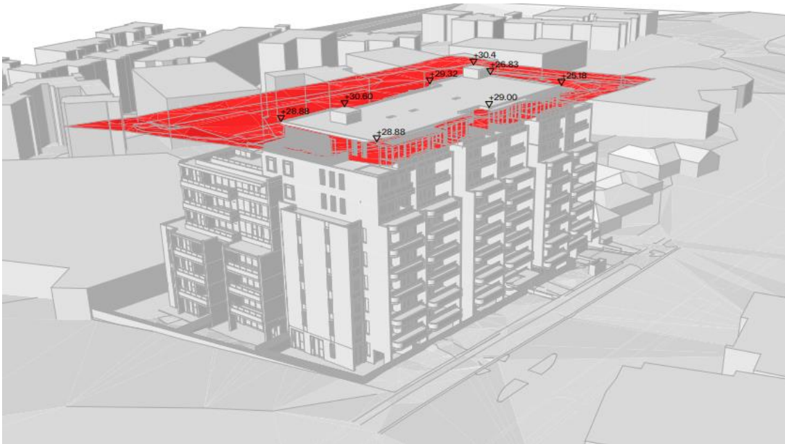
Figure 23: Building height envelope (Source: PBD Architects)
