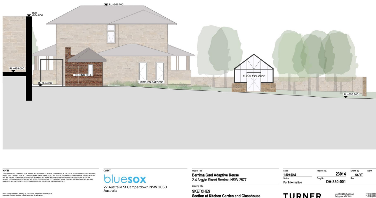
Figure 4 – Elevation of Glasshouse
