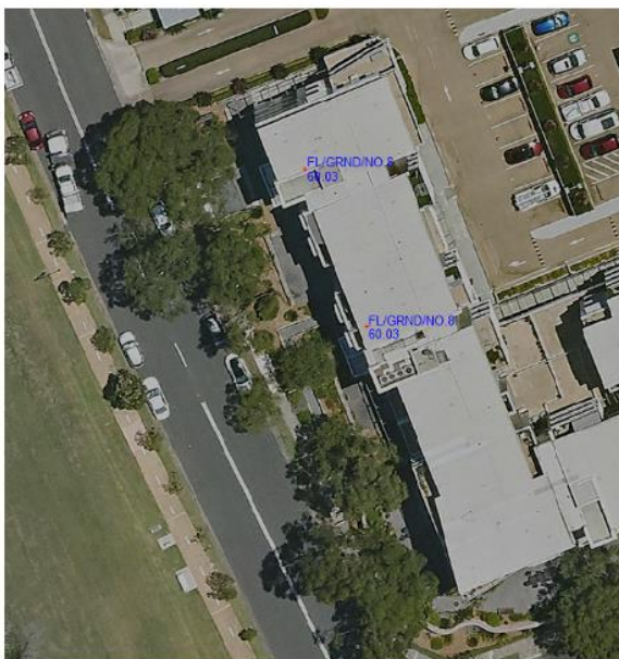
Figure 21 - Ground Floor Level Surveys of No. 2 Free Settlers Drive (By Registered Surveyor, Orion 11/02/2026)
