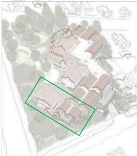
Figure 14 How the varied roof pitches of the existing building were used to influence the form of the new additions (Source: PBD Architects)
