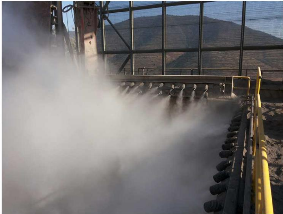
Figure 1 - Fine Mist Spray on a Dump Hopper
