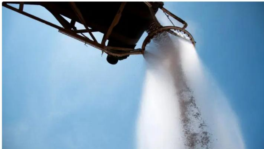
Figure 5 - Water Mist Dust Suppression at Stockpile
