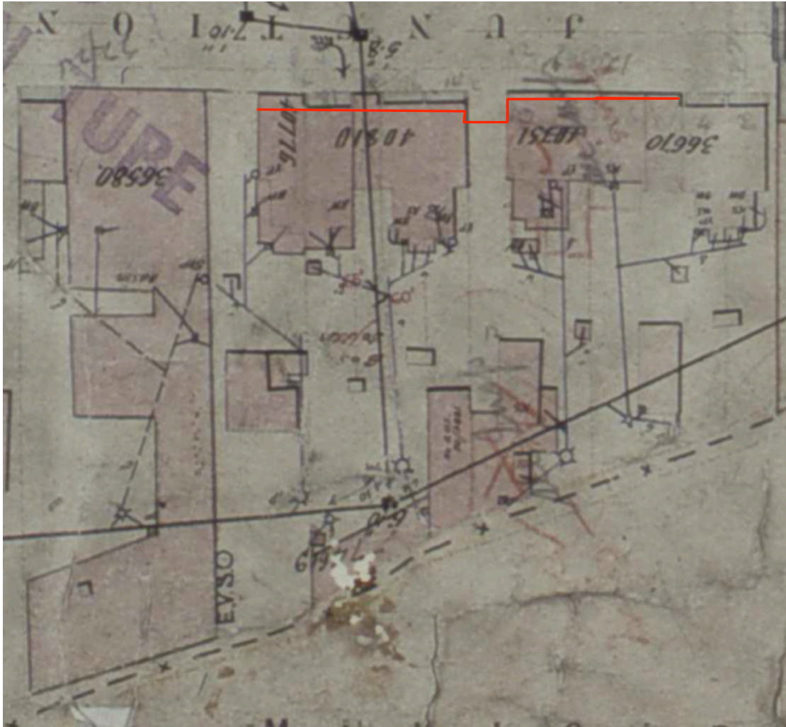
CMP Figure 5.3 J.F. Truscott, Blackwattle Detail Series, The Glebe, Sheet 3 1, June 1889. Detail only with approximate line of wall highlighted. No wall is shown on the open area between the buildings where the current wall steps in
