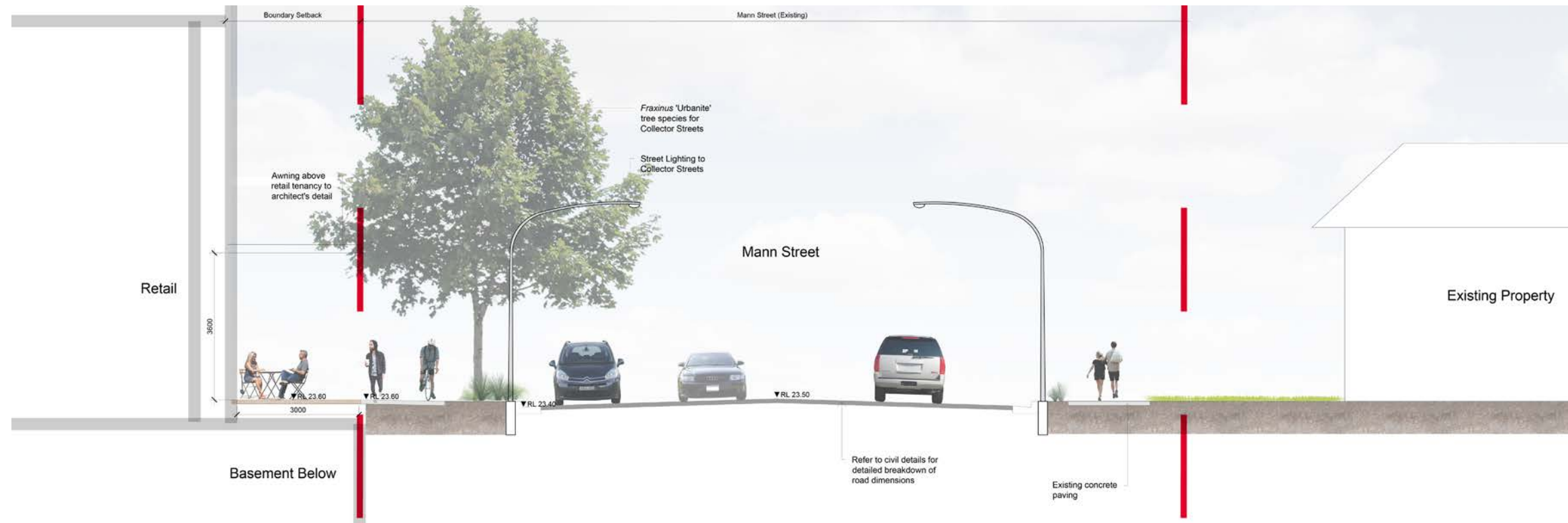
Mann Street - Proposed Site Condition Section A-A
