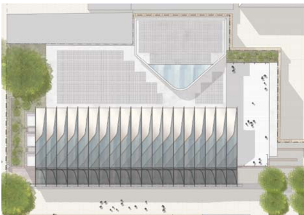
Figure 199: Roof plan – showing photovoltaics
