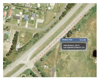
Turning Right from the Federal Highway to Collector Road – deceleration lane is 225 m
