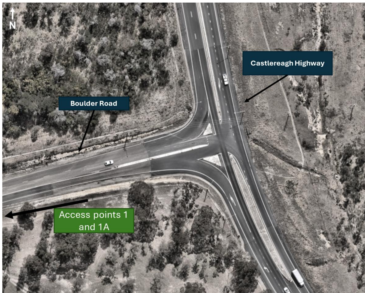
Figure 4.11 Boulder Road / Castlereagh Highway intersection layout
