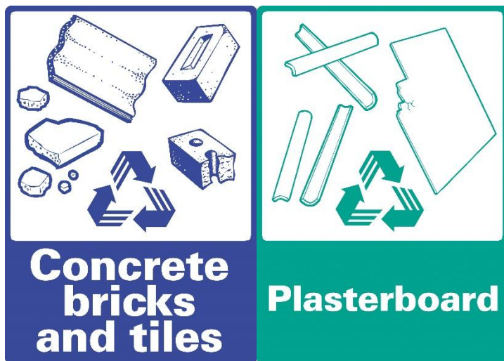
Figure 4-2: Example signage for construction waste bins
