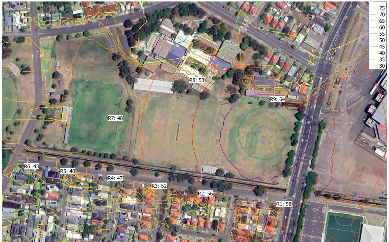
Figure 4-2 Construction Excavation East dB(A) Leq(15min)
