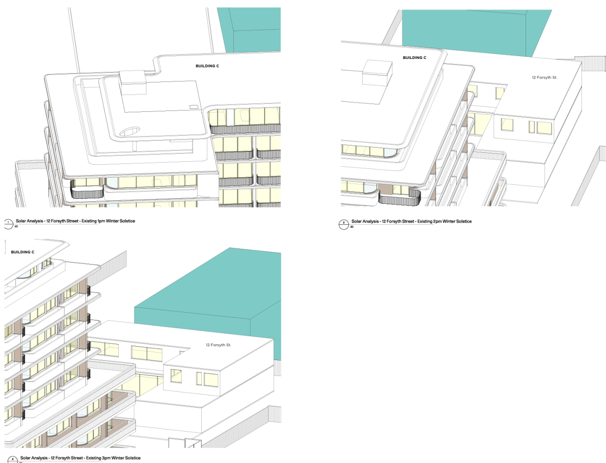
Figure 35 View from the sun showing 12 Forsyth Street between 1pm and 3pm (Source: PMDL)
