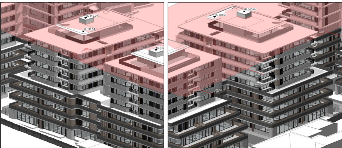
Figure 5 Building height plane of building B when viewed from the north-east (left) and north-west (right) (Source: PMDL Architects)
