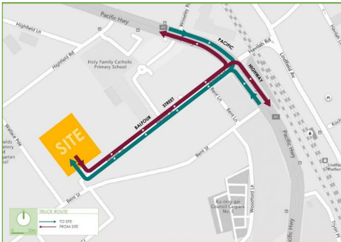
Figure 6: Structure and Fitout Truck Routes
