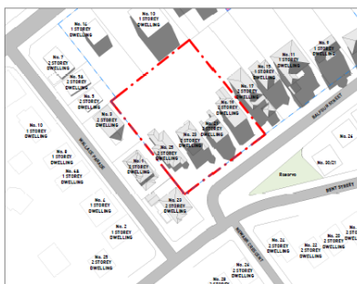
3 OVERSHADOWING - 01.30PM JUNE 21 (EXISTING) 1 : 1000
