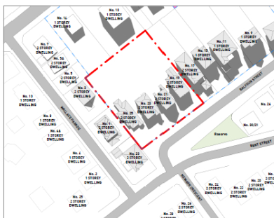
1 OVERSHADOWING - 01PM JUNE 21 (EXISTING) 1 : 1000
