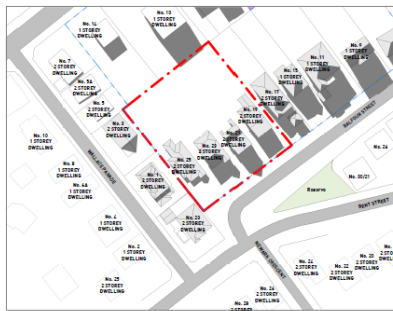
1 OVERSHADOWING - 02PM JUNE 21 (EXISTING) 1 : 1000
