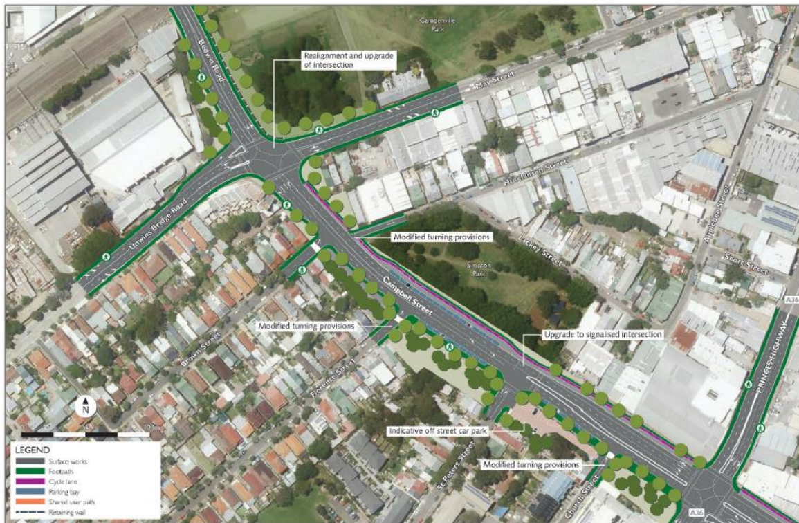
Figure 5-31 Bedwin Road, Campbell Street and Campbell Road realignment, widening and extension works - map 1
