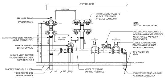
DN150 FIRE HYDRANT BOOSTER ASSEMBLY DETAIL
