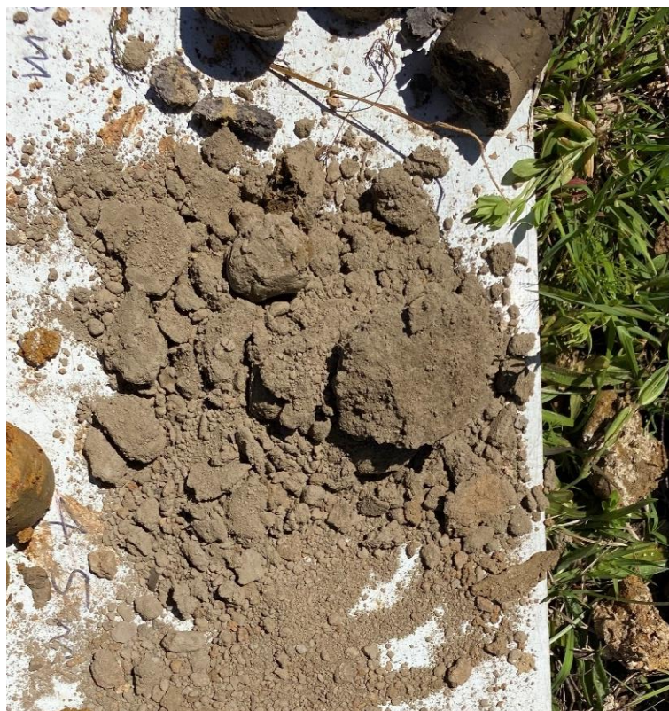
Photo 10: Typical Photo of Deep FILL Unit at Regional Basin Bund Weir
