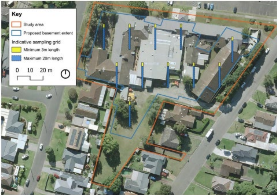
Figure 3.1 Indicative 20m x 20m sampling grid. (Source: Six Maps with GML overlay)
