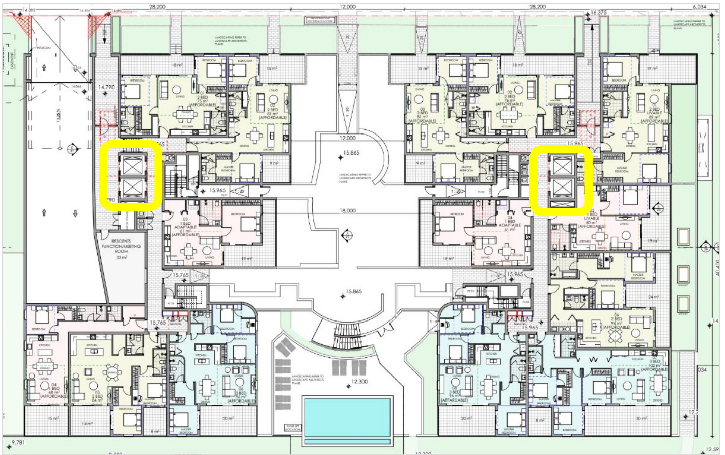
Figure 3: Amended typical floor plan with 2 lifts per envelope outlined yellow (Source: PTI/PPUD)
