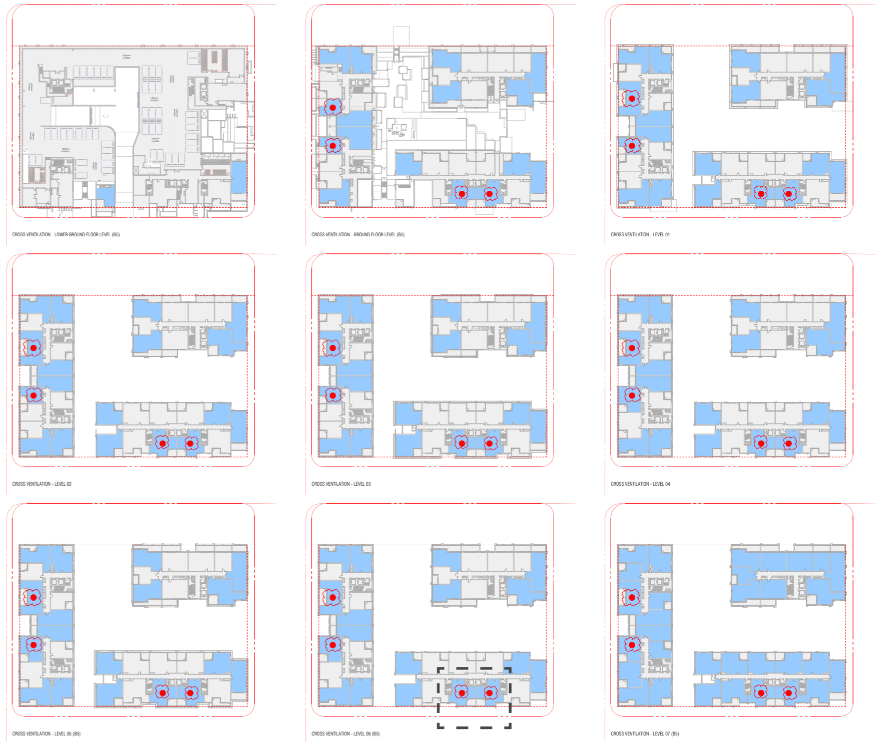
DA-E-B5-AR-503 COMPLIANCE - CROSS VENTILATION
