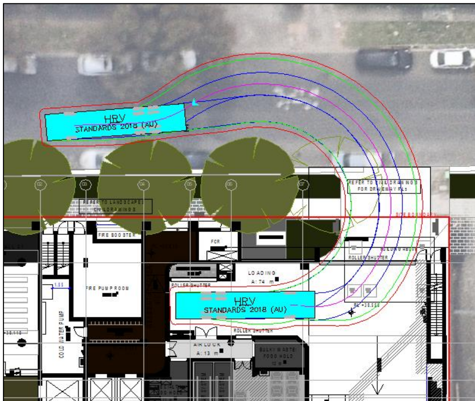
12.5M LENGTH HRV – SITE ACCCES, SITE EGRESS AND LOADING [2] SUCCESSFUL – 2 Manoeuvres Reverse IN, 1 Manoeuvre Forward OUT
