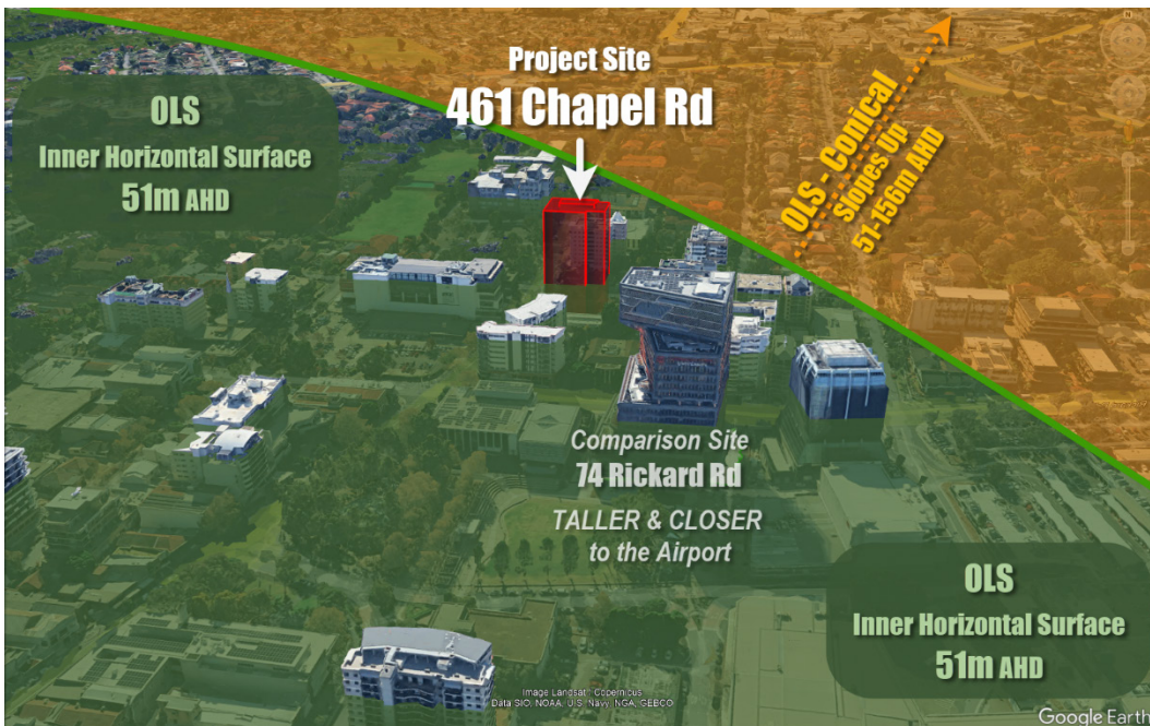
Figure 4-2 — Site in relation to Bankstown Airport's OLS & Nearby Taller Buildings (in 3D)
