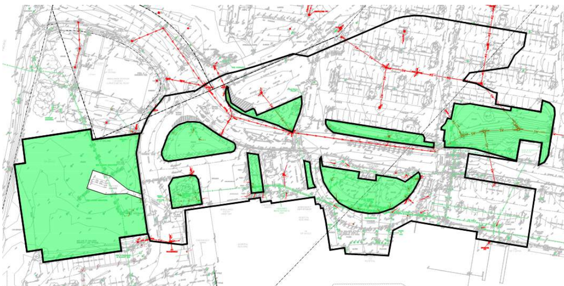
Figure 3 Existing Development site catchment areas ultimately draining to pit H1 (existing pervious and impervious proportion)
