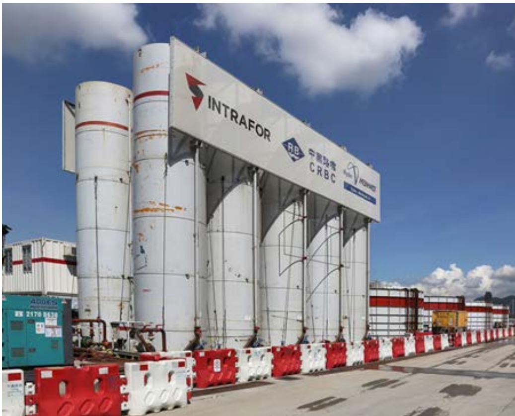
Figure A2-2 A bentonite plant with storage silos indicative to the requirement for the President Avenue construction ancillary facility
