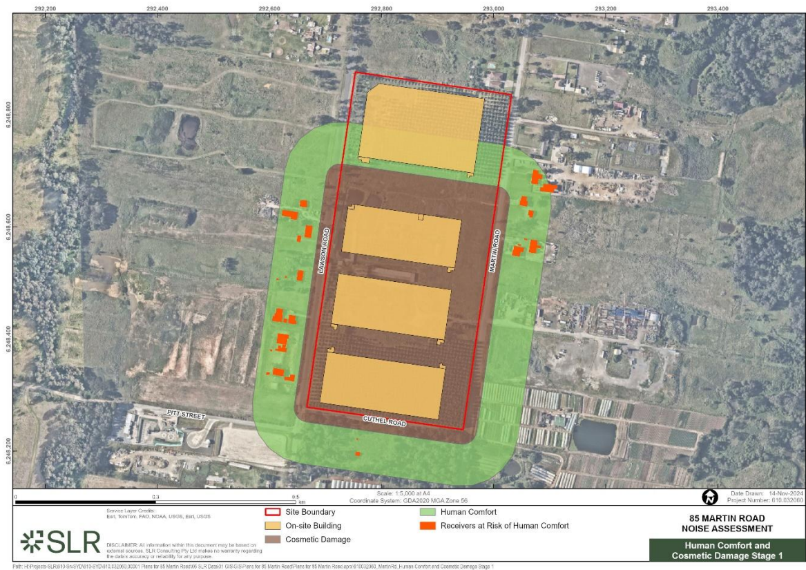
Figure 8 Construction Vibration – Large Vibratory Roller
