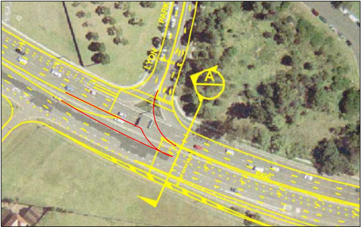
Figure 6: Proposed Lyonpark Road / Epping Road layout
