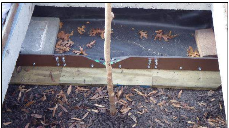
Figure 22. Inflow compound weir for flow measurement
