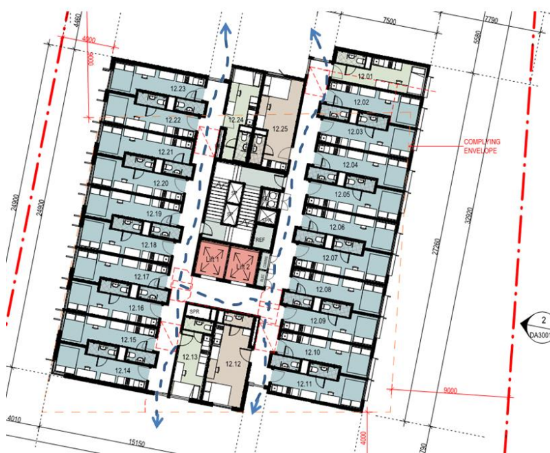
Figure 7 Proposed Naturally Ventilated Common Corridors - Typical Floor Plan
