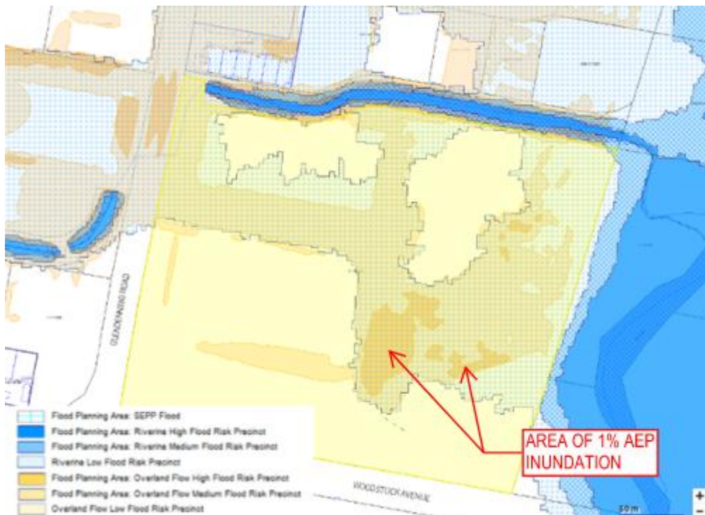
Figure 1. Blacktown Council Flood Maps – 1% AEP Extent of Inundation to Subject Site (Medium Flood Risk Precinct) – Existing (Pre-Development) Scenario
