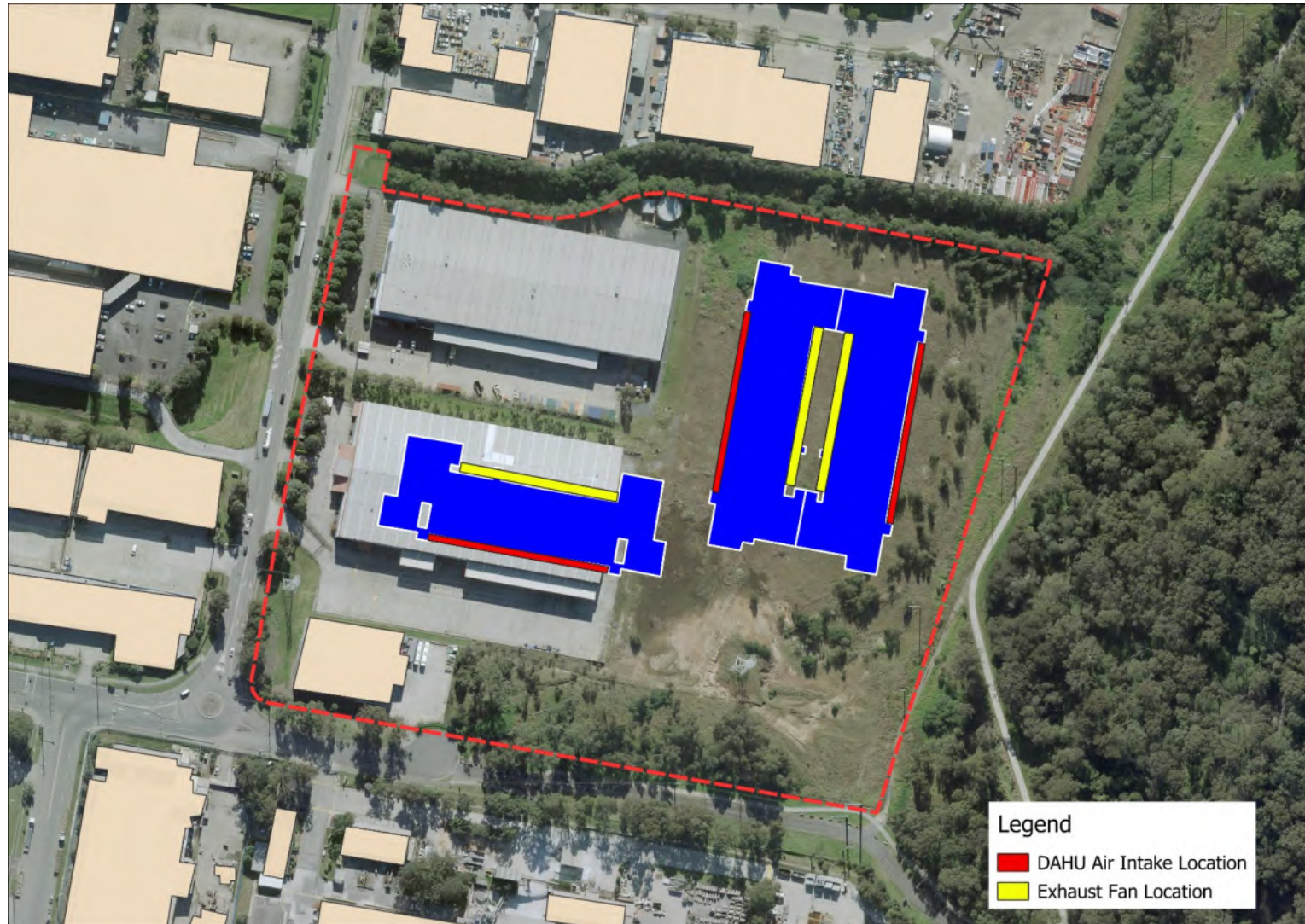
Figure 14 Operational scenario 04 - modelled mechanical noise emission sources visualised for the Day / Evening / Night Period.
