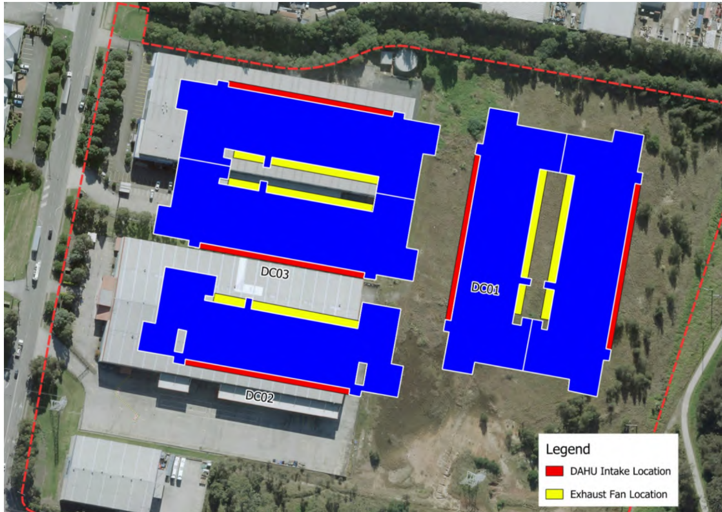
Figure 12 Operational scenario 01 & 02 - modelled mechanical noise emission sources visualised for the Day / Evening / Night Period.
