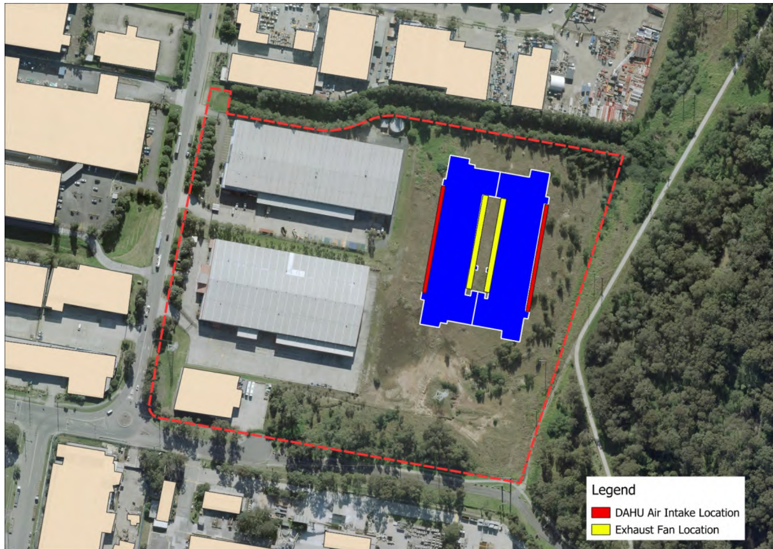
Figure 13 Operational scenario 03 - modelled mechanical noise emission sources visualised for the Day / Evening / Night Period.
