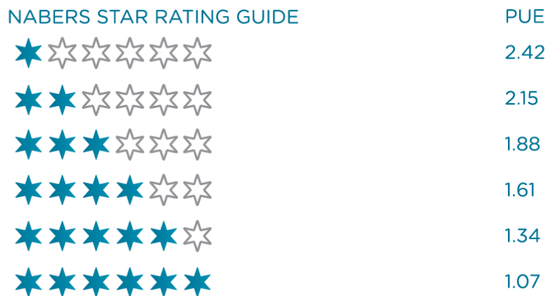
Figure 12: How NABERS star ratings correspond to PUE values (Source: Data Centres | NABERS )
