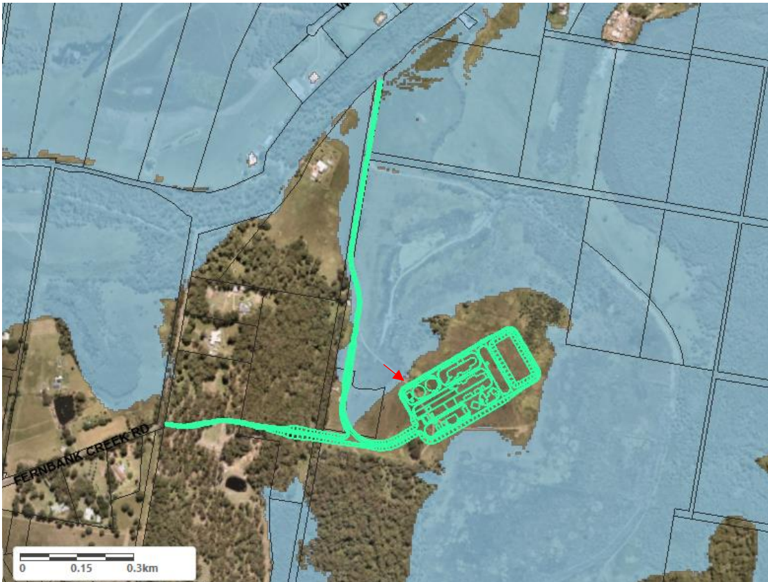
Figure C.3 The proposed Thrumster Wastewater Treatment Plant and access roads layout relative to the May 2025 flood peak extent
