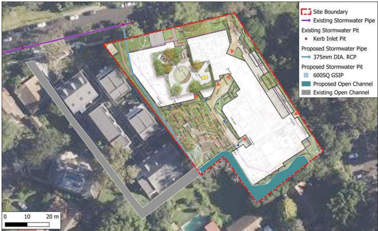
Figure 6 Modelled Stormwater Infrastructure
