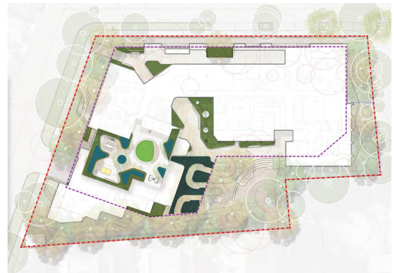
Figure 13: On structure soil depth plan
