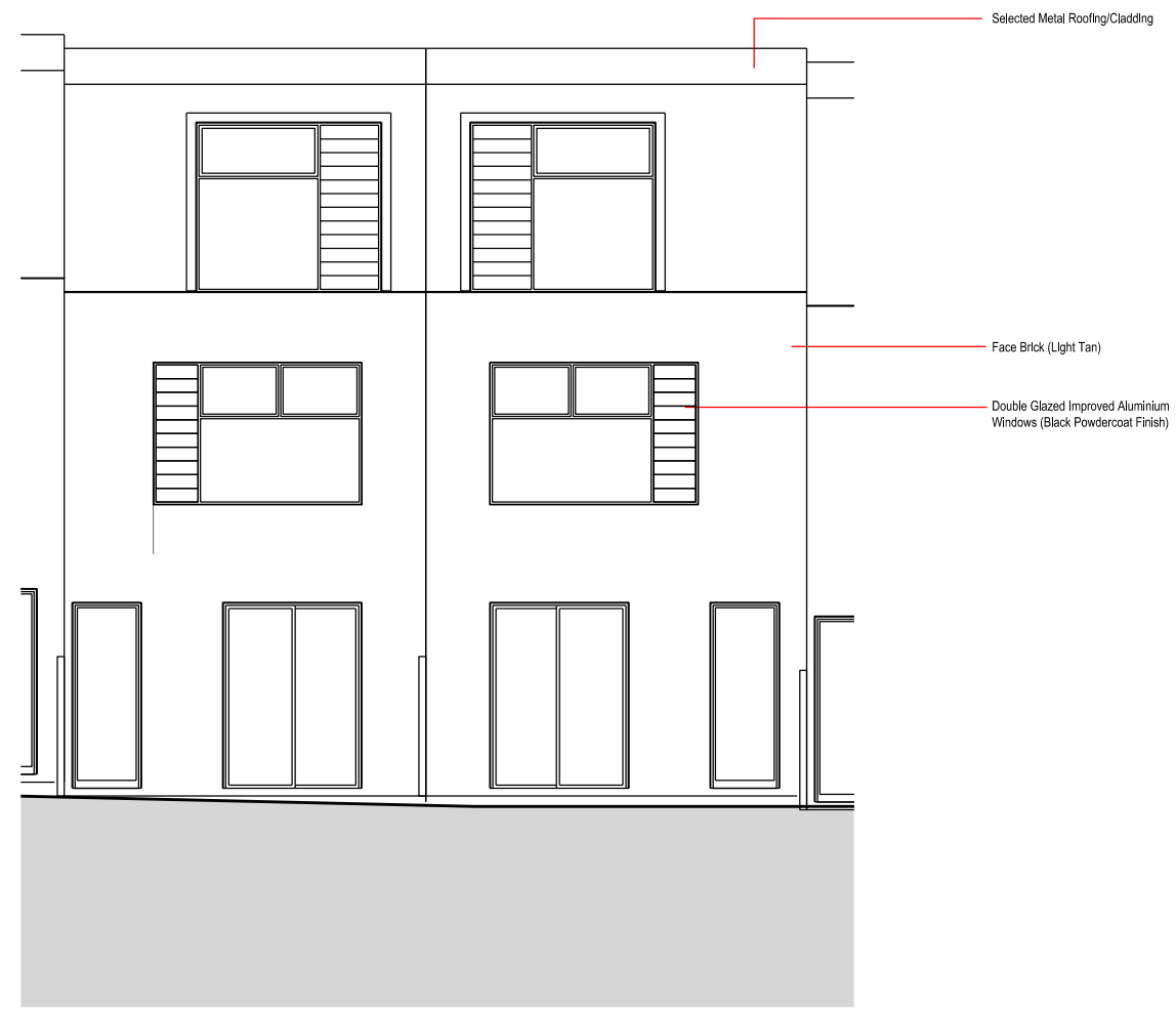
Typical Unit East (Rear) Elevation
