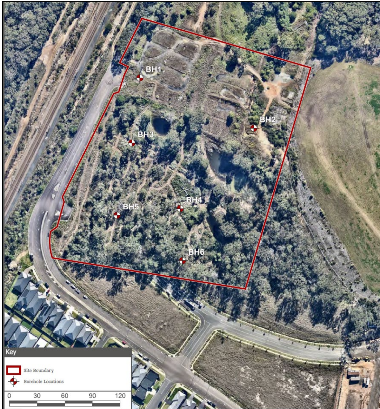
Figure 3 – Geotechnical Borehole Locations
