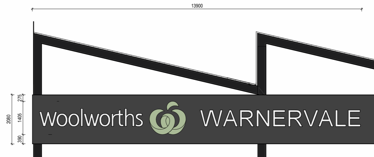
S9 WOOLWORTHS SIGN INTERNALLY ILLUMINATED WOW SIGN. SINGLE SIDED ON SOLID BLACK SOLID BACKING. REFER TO WOOLWORTHS SIGNAGE GUIDELINES
