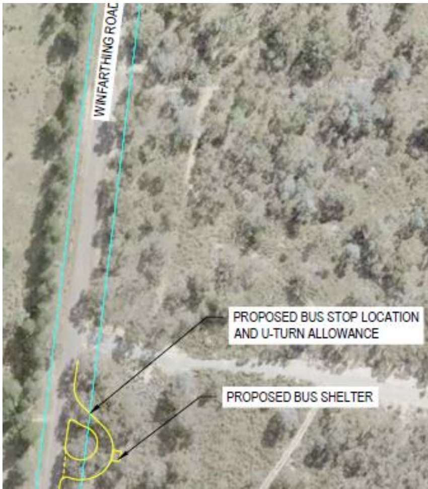
Figure 3.1 Bus stop and turning circle arrangement
