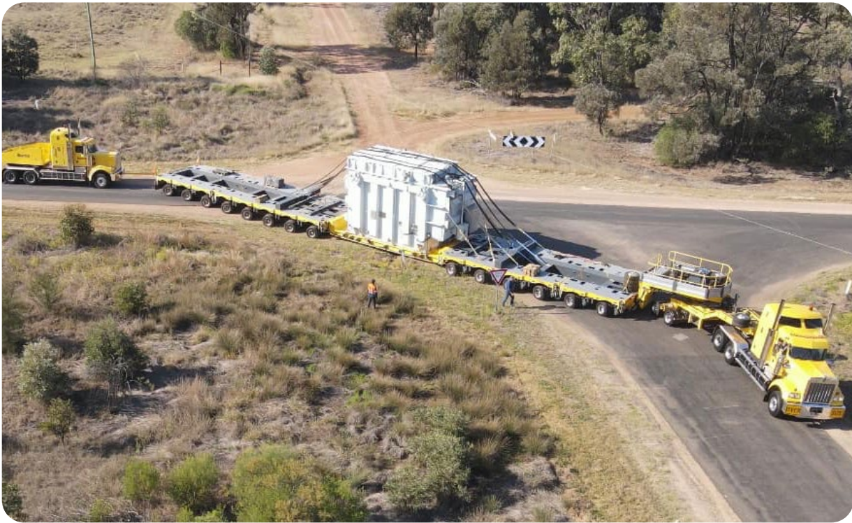
Above: ARES transporting a 170-ton transformer on a custom drop frame trailer. Below: Schematic of proposed trailer for Gundry SF.
