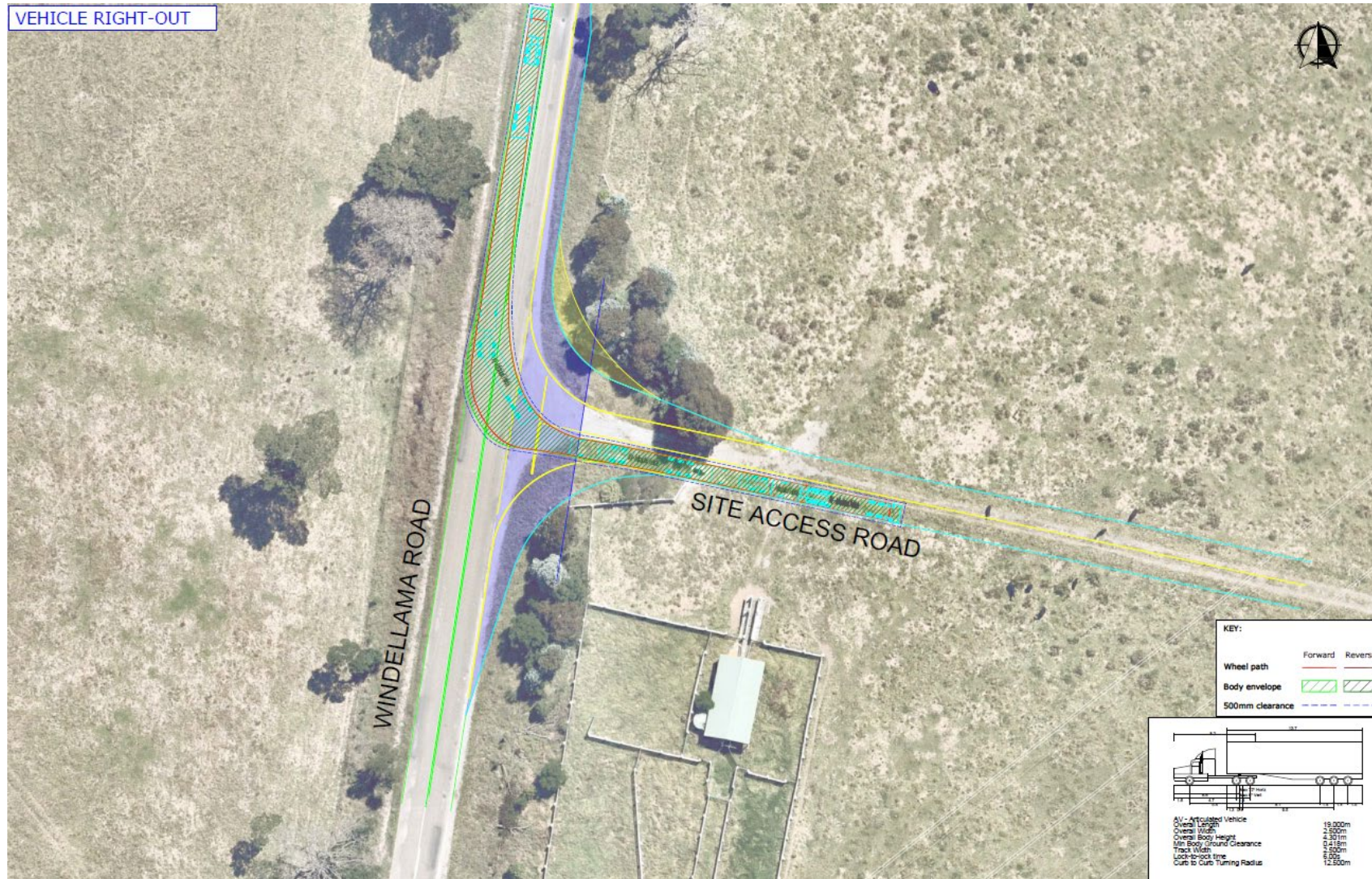
Figure 5.4: 19m Semi Trailer Swept Path (Exit) – Project Site Access at Windellama Road
