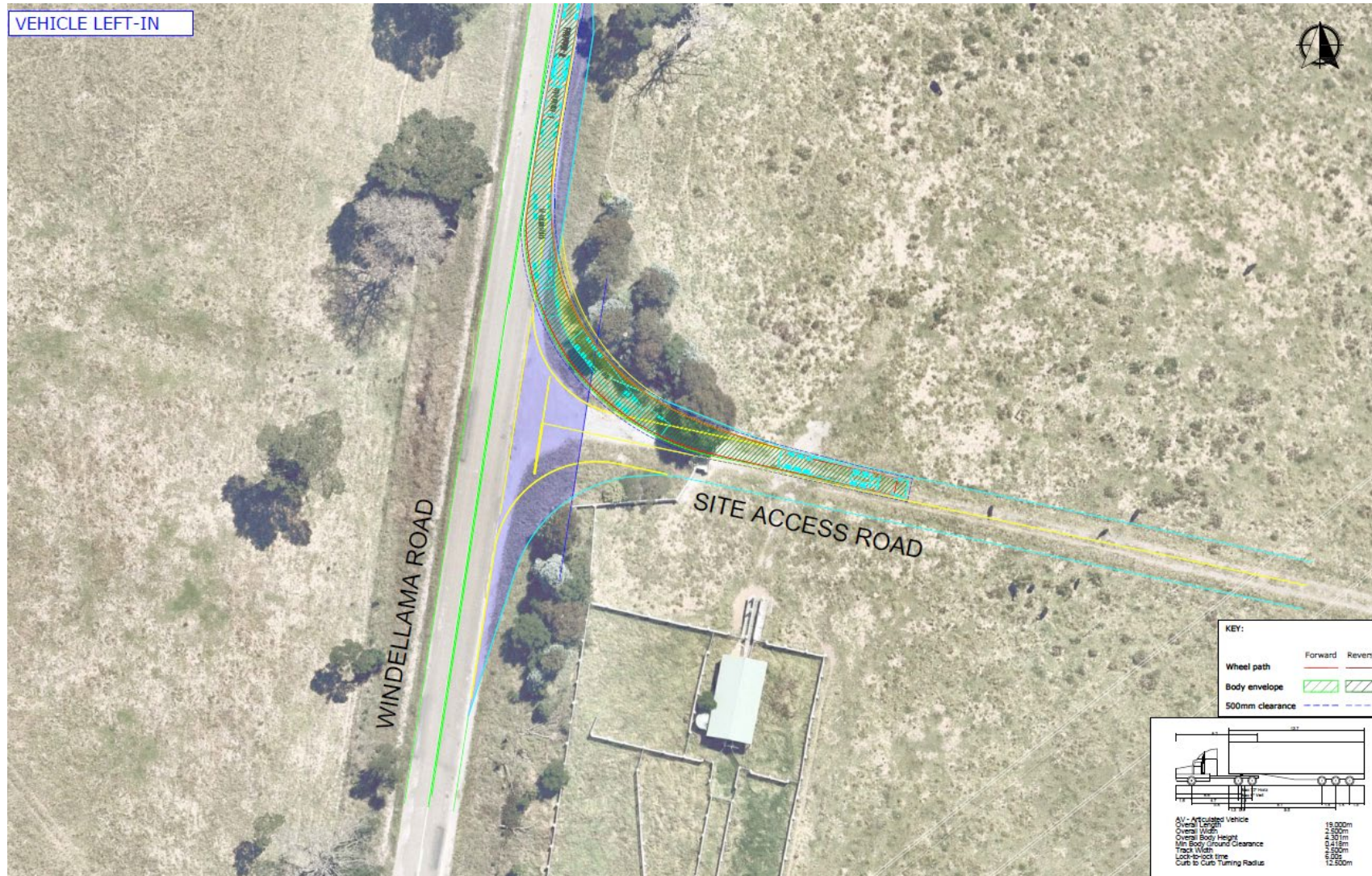
Figure 5.3: 19m Semi Trailer Swept Path (Entry) – Project Site Access at Windellama Road
