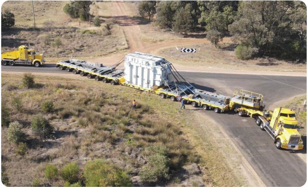
Figure 4.1: Typical OSOM Vehicle Transporting Transformer (47.5m long)
